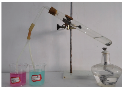
Fig. 1 The gas product testing device for reaction of concentrated sulfuric acid and zinc particles
