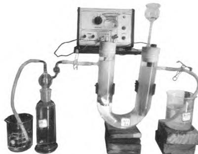
Fig. 4 Gas generated in both anode and cathode after electrolysis
